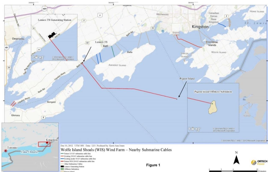
Figure 10-3: Kingston area Submarine Cable Installations
