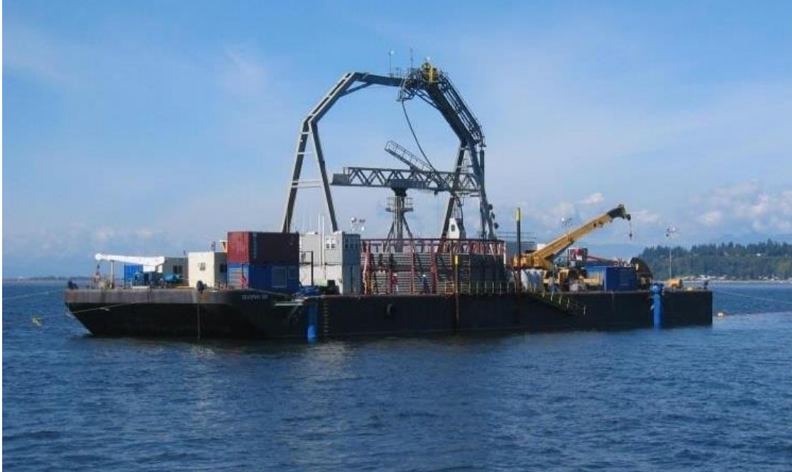
Figure I-29: Cable Installation Barge (Courtesy of Caldwell Marine)
