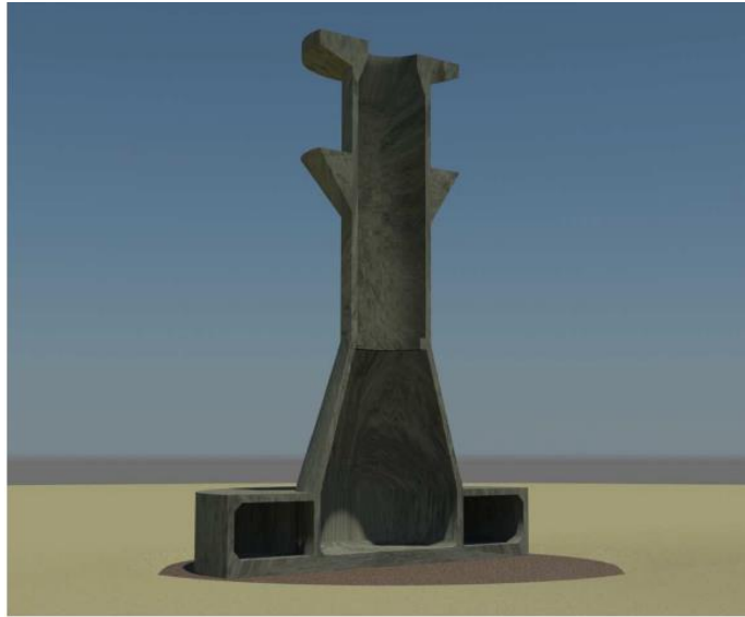
Figure 8-2: Cross Section of Semi-Floating Gravity Base Foundation
