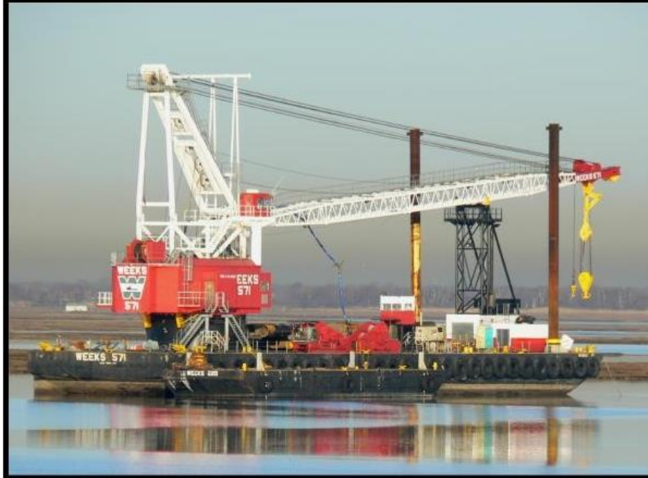
Figure G-15: Weeks 571 Barge for Dredging and Bedding Stone Placement
