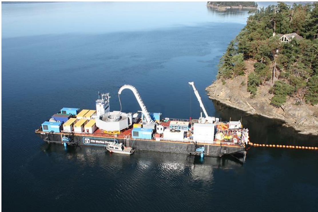
Figure I-29: Cable Installation Barge (Courtesy of Caldwell Marine)
