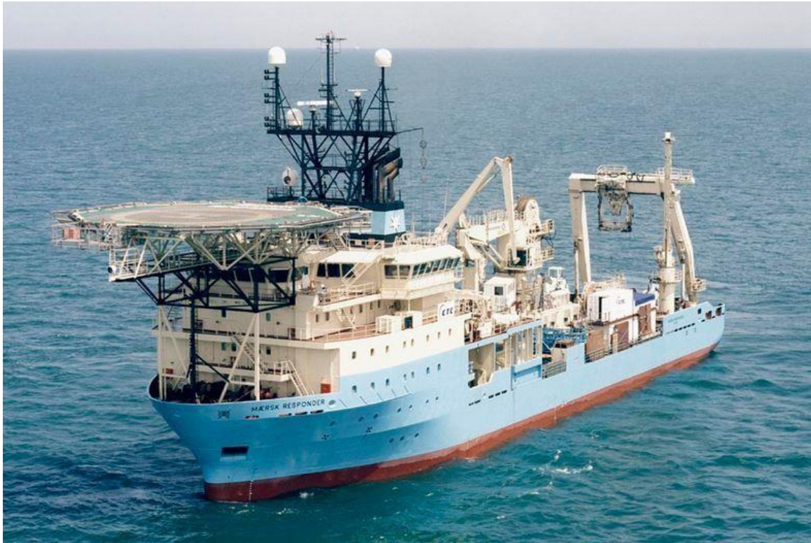
Figure I-31: Cable Installation Vessel (Courtesy of Maersk)
