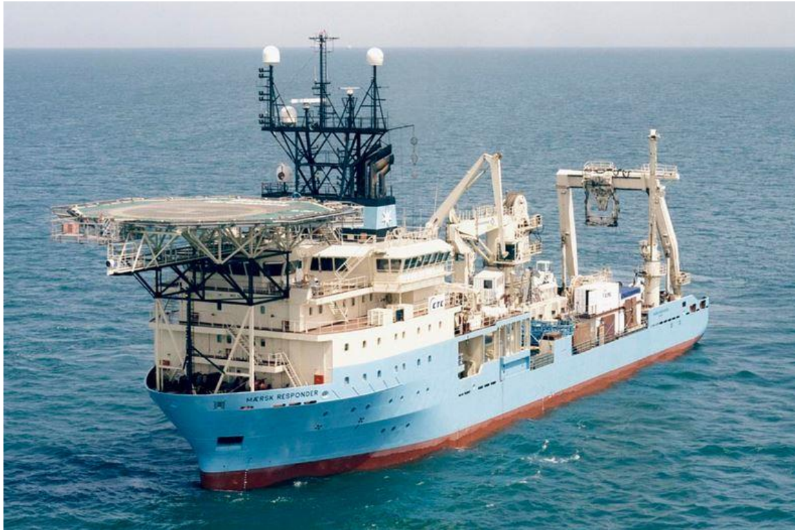
Figure 10-7: Cable Installation Vessel 12
