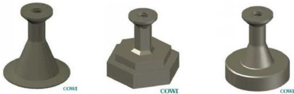
Figure 8-1: Gravity Base Foundation Designs
