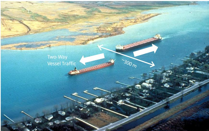
**Figure 5.9: St. Clair River Channel, showing two-way vessel traffic in 300 m wide channel**
