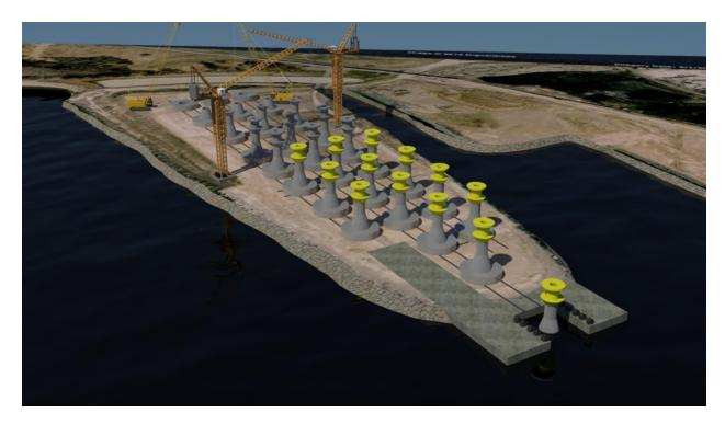
Figure A.32 - Fabrication Facility with Foundation in Launch Position
