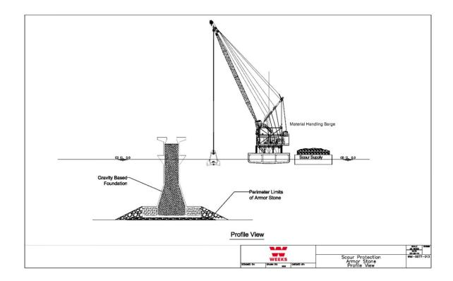
Figure A.43 - Scour Protection - Profile View
