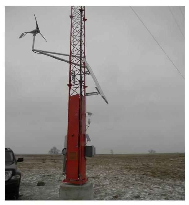
Figure A.10 - Solar Panels, Wind Turbine, Battery Bank, Logger Enclosure, Satellite
