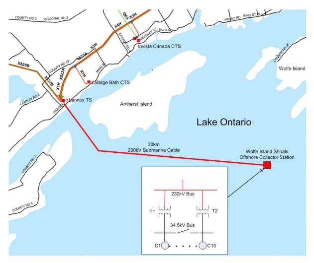
Figure A.51 - Approved Connection between Wolfe Island Shoals (offshore) substation and Lennox (onshore) Generating Station
