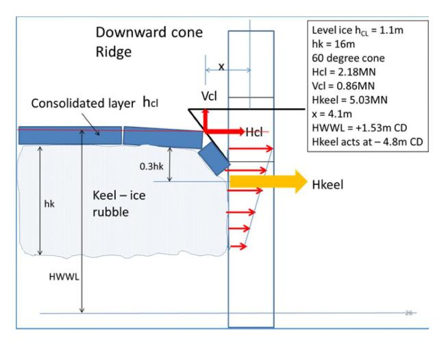
Figure A.64 - LEEDCo Icebreaker Ice Loading on Turbine Foundation, Lake Erie
