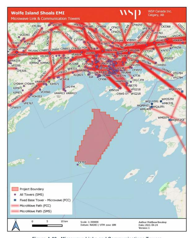
Figure A.83 - Microwave Links and Communications Towers
