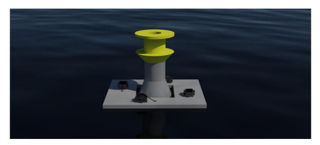
Figure A.36 - Semi Floating Gravity Foundation with Supplemental Floatation
