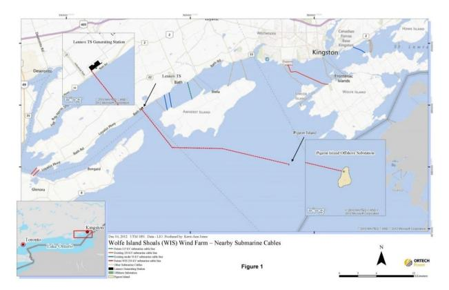
**Figure A.49 - Kingston Area Submarine Cable Installations**
