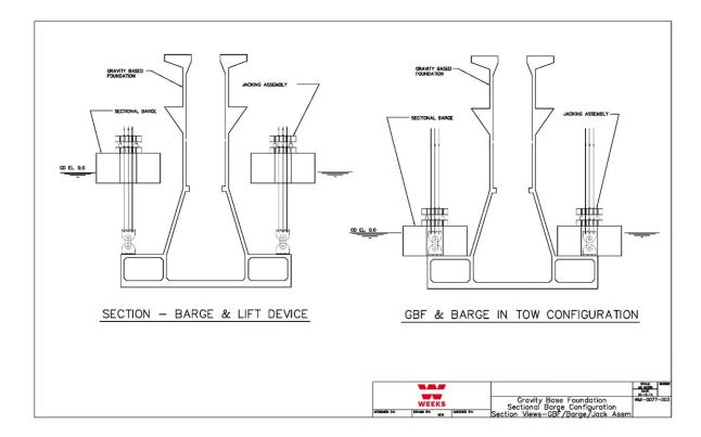
Figure A.35 - Jacking Assembly - Section Views
