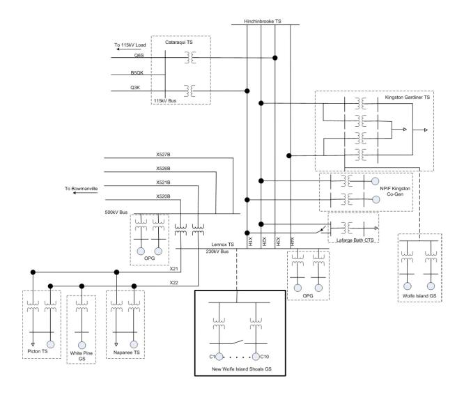
Figure A.52 - Hydro One Transmission System and Wolfe Island Shoals Electrical
