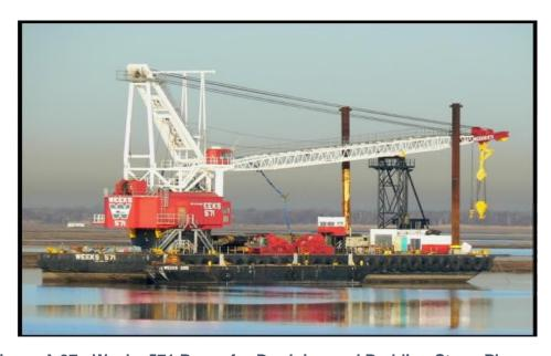
Figure A.37 - Weeks 571 Barge for Dredging and Bedding Stone Placement
