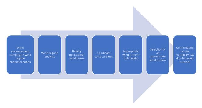
**Figure A.4 - Wind Turbine Selection Process**
