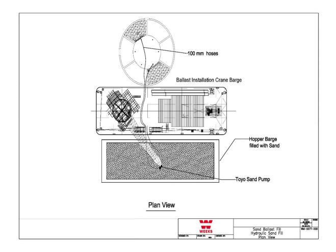
Figure A.38 - Hydraulic Sand Ballast - Plan View
