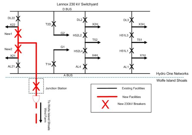
Figure A.53 - Wolfe Island Shoals Point of Connection in the Lennox 230kV Switchyard
