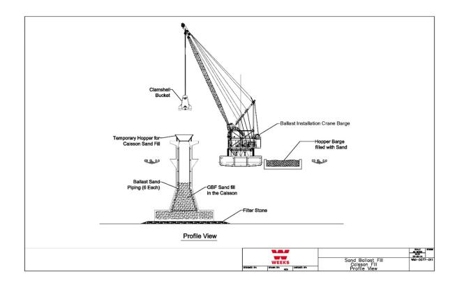
Figure A.41 - Mechanical Sand Ballast - Profile View
