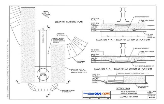
Figure A.33 - Foundation Elevator Detail
