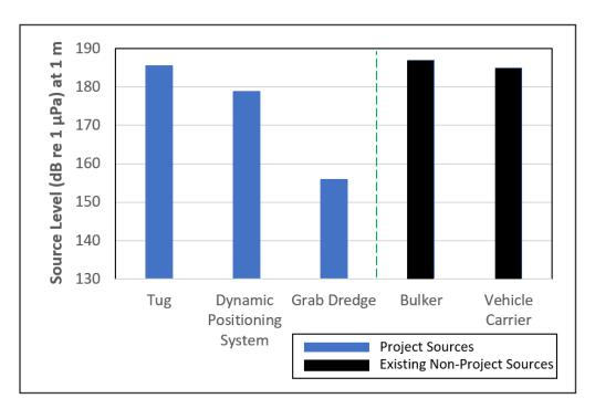
Figure A.77 - Noise Emissions of the Various Project Noise Sources Relative to Existing Non-Project Noise Sources in the Vicinity
