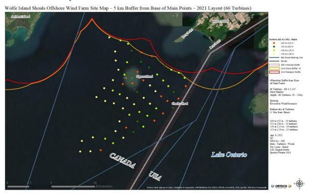
Figure A.1 - Project Layout Showing 5km Setback
