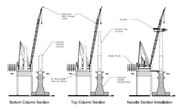
Figure A.45 - Wind Turbine Tower and Nacelle Installation
