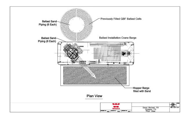
Figure A.40 - Mechanical Sand Ballast - Plan View
