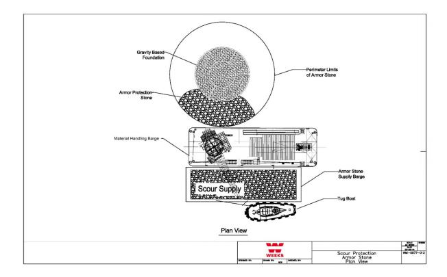
Figure A.42 - Scour Protection - Plan View
