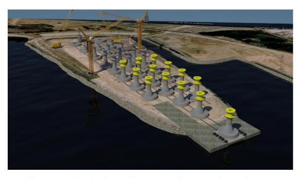
Figure A.31 - Fabrication Facility Layout with Foundation on Elevator
